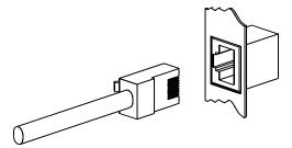
Figure 2-4. Inserting a loop-back plug into an RJ-45 port
